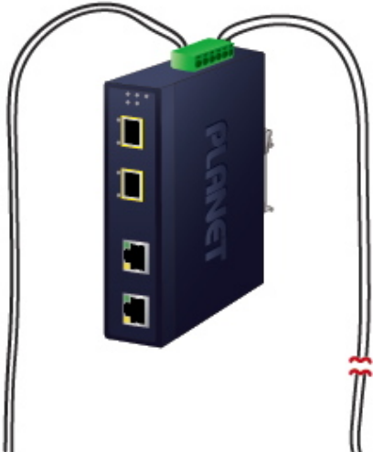
DC Power Failure
